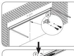
Mount the door bracket (3), on the door's centre line one-third down the top panel and mounted using M6 or equivalent screws (not supplied), STEEL DOORS ONLY: Bracket can be
